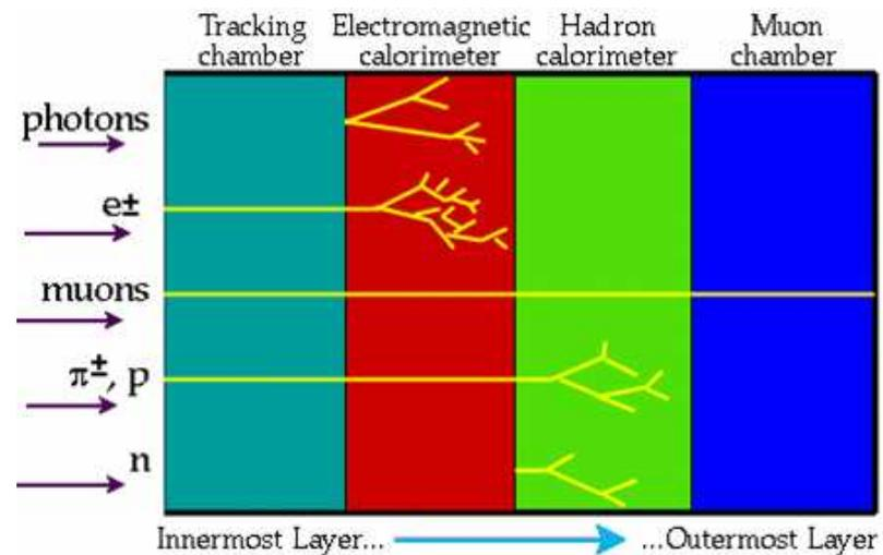
A detector consists of tracking systems, calorimeters, muon systems to identify various particles.
